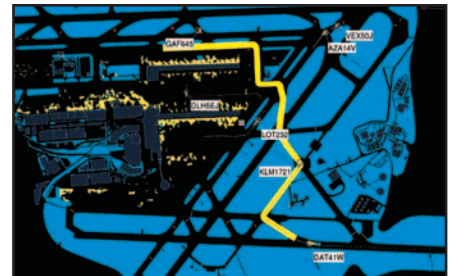
Ground Radar Data Display (GND RDD)
